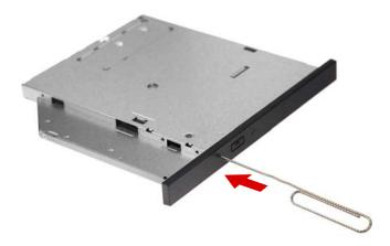
6. Disengage the latch securing the ODD bezel to the ODD tray and detach the bezel from the ODD module.
