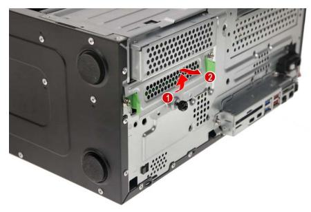
7. Slide the HDD2 carrier out of the chassis.
