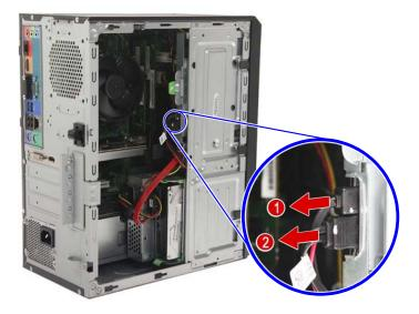
2. Press the retaining latch and slide the ODD module out of the chassis.
