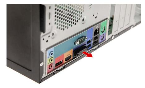
4. Remove the eight screws securing the mainboard to the chassis.
