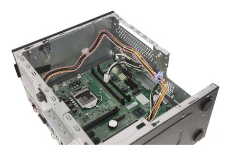
3. Remove the two screws securing the rear end of the power supply module to the chassis.
